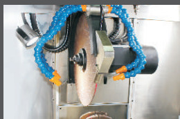
Cut off wheel cooling systems
